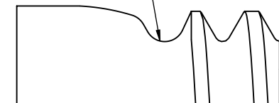
VIEW A HI-LITE™ THREAD TRANSITION AREA. SEE SPECIFICATION FOR INSPECTION
