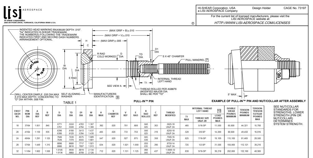
GENERAL NOTES: 1. Concentricity: "A" to "D" diameter within .010 FIM. 2. Dimensions in inches and to be met after finish. ② 3. Surface texture per ASME B46.1.
