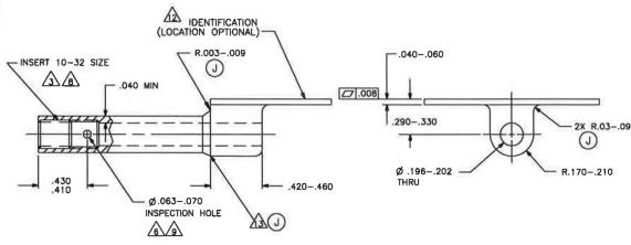
14. PART NUMBER EXAMPLE: 5300019-()()()()() NO SUFFIX = WITH INSPECTION HOLE "NH" SUFFIX = NO INSPECTION HOLE HELICAL COIL INSERT FINISH OPTIONS /3 NO SUFFIX = INSPECTION HOLE NOT DEBURRED "C" SUFFIX = INSPECTION HOLE DEBURRED MOUNTING HOLE OPTIONS /7 - LENGTH OPTIONS
